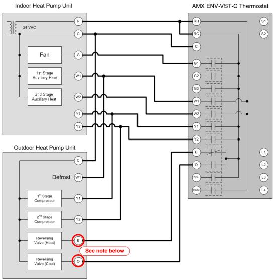
FIG. 9 Two Stage Heat Pump wiring
